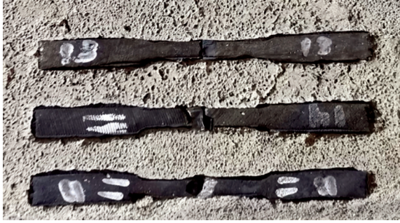
Fig. 3. Failure specimens after vacuum furnace brazing with 5 min bonding time.
